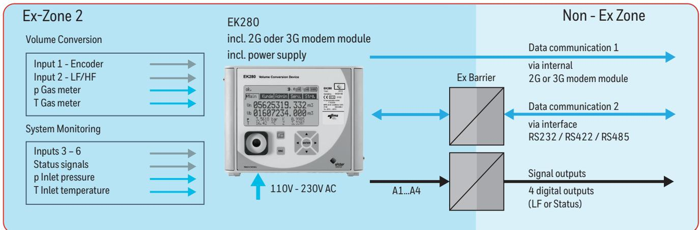
The system installer is responsible for completing the installation. Explosion protection must be given due consideration when connecting intrinsically safe devices.
