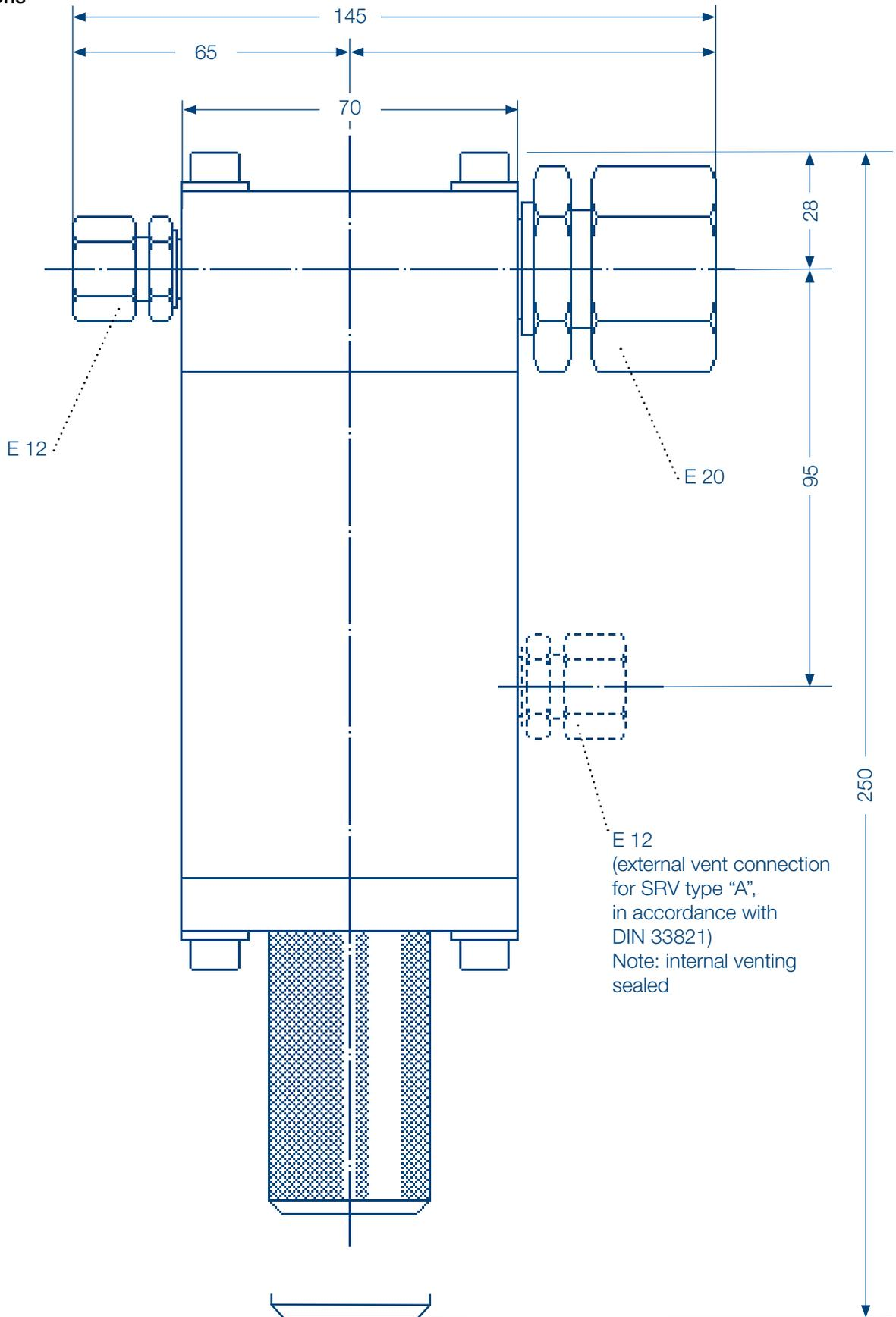
A safety relief valve (SRV) has the task of autonomously releasing a gas flow from a pressurised line, as soon as the pressure in the system to be safeguarded reaches the set response pressure through increasing increments. The SRV closes again when the pressure in the system to be safeguarded drops below the closing pressure.
